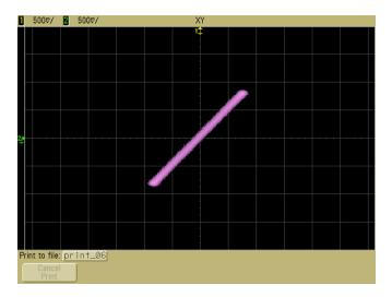
Figure 21 Signals are in phase
