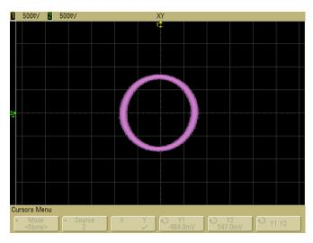
Figure 20 Signals are 90 out of phase
