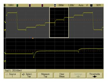
Figure 35 Isolating area for Top measurement
