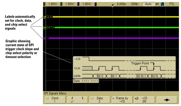
**4** Press the **Data** softkey or turn the Entry knob to select the channel that is connected to the SPI serial data line. The
