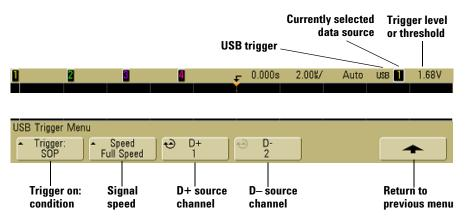
**2** Press the **Speed** softkey to select the speed of the transaction being probed.
