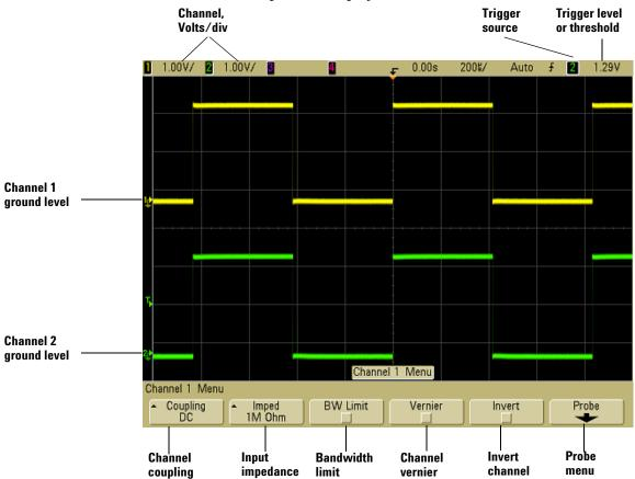
Pressing an analog channel key displays the channel's menu and turns the display of the channel on or off. The channel is displayed when the key is illuminated.
