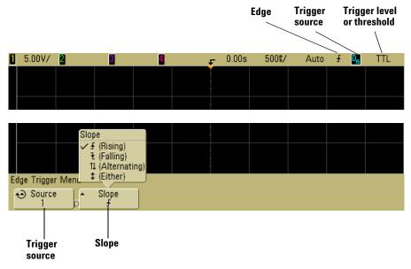
**2** Press the **Slope** softkey and select rising edge, falling edge, alternating edges, or either edge. The selected slope is displayed in the upper-right corner of the display.
