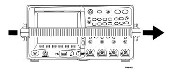
**2** Without releasing the hubs, rotate the handle to the desired position. Then release the hubs. Continue rotating the handle until it clicks into a set position.
