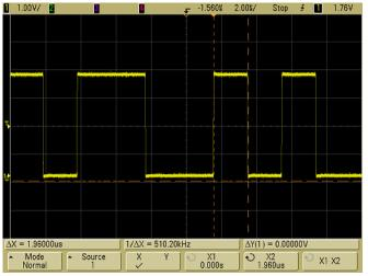
Put the X1 cursor on one side of a pulse and the X2 cursor on the other side of the pulse.
