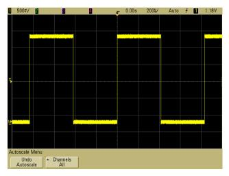
If you see the waveform, but the square wave is not shaped correctly as shown above, perform the procedure "To compensate the oscilloscope probes" on page 23. If you do not see the waveform, ensure your power source is adequate, the oscilloscope is properly powered-on, and the probe is connected securely to the front-panel oscilloscope channel input BNC and to the Probe Comp terminal.
