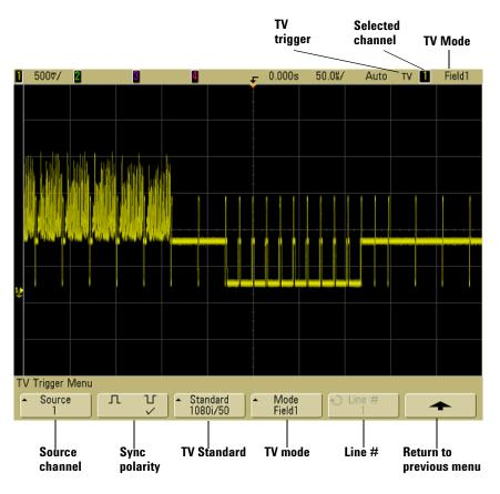
in the **Trigger** softkey, then press the **Settings** softkey to display TV trigger menu.
