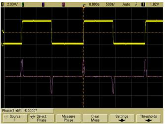
The example below shows a phase measurement between the channel 1 and the math d/dt function on channel 1.
