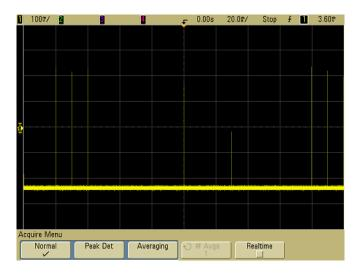
Figure 41 15 ns Narrow Pulse, 20 ms/div, Normal Mode
