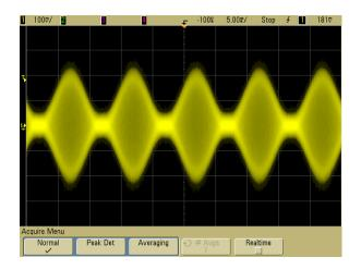
Figure 38 Amplitude Modulation with Noise Shown at 40% Intensity
