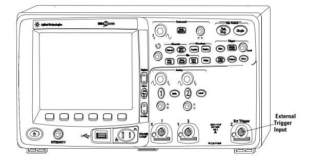
Figure 26000 Series 2-Channel Oscilloscope Front Panel
