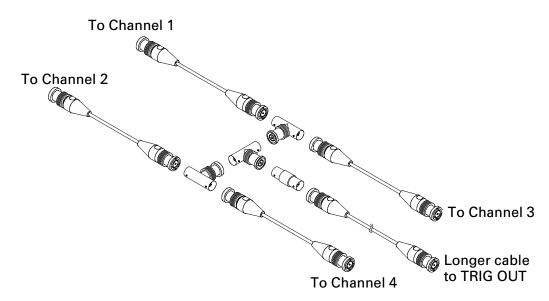
Figure 6 User Calibration cable for 4-channel oscilloscope
