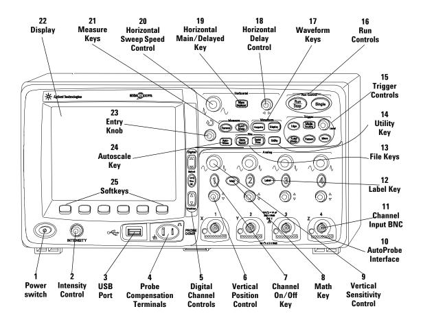
Figure 16000 Series 4-Channel Oscilloscope Front Panel
