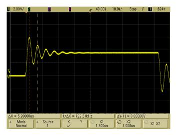
Figure 29 Cursors measure frequency of pulse ringing
