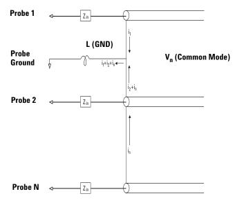
Figure 46 Common Mode Input Voltage Model
