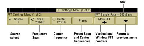
**Source** selects the source for the FFT. The source can be any analog channel, or math functions 1 + 2, 1 - 2, and 1 \* 2.
