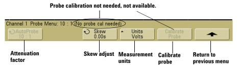
**Probe Attenuation** If you have a self-sensing probe (such as the 10073C or 10074C) connected to the analog channel, the oscilloscope will automatically configure your probe to the correct attenuation factor. In this case, you can not change the probe attenuation factor. In the previous figure, the oscilloscope has sensed an AutoProbe 10:1 probe.
