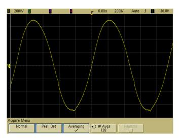
Figure 40 128 Averages used to reduce random noise
