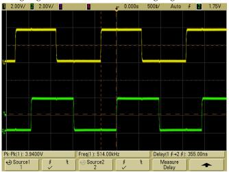
The following example shows a delay measurement between the rising edge of channel 1 and the rising edge of channel 2.
