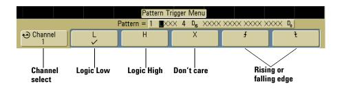
**2** For each analog or digital channel you want to include in the desired pattern, press the **Channel** softkey to select the channel.
