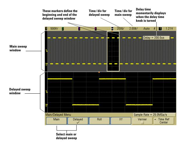
The area of the main display that is expanded is intensified and marked on each end with a vertical marker. These markers show what portion of the main sweep is expanded in the lower half. The Horizontal knobs control the size and position of the delayed sweep. The delay value is momentarily displayed in the upper-right portion of the display when the delay time  $(\blacktriangleleft)$  knob is turned.
