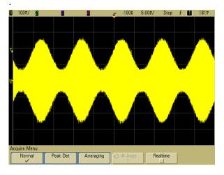
**Figure 37** Amplitude Modulation with Noise Shown at 100% Intensity
