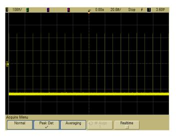
Figure 42 15 ns Narrow Pulse, 20 ms/div, Peak Detect Mode
