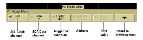
**2** Connect an oscilloscope channel to the SCL (serial clock) line in the circuit under test, then set the **SCL** clock channel softkey to that channel.
