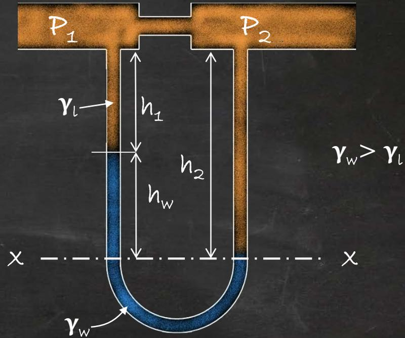
$$P_1 + \gamma_l h_1 + \gamma_w h_w = P_2 + \gamma_l h_2$$
