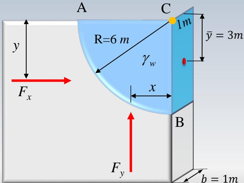
$$F_x = \gamma_w \bar{y} A_{CB} = 9810 \times 3 \times (6 \times 1)$$
