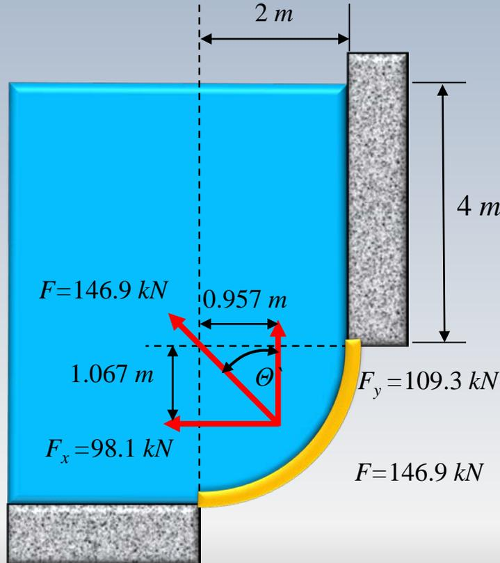
$$F_x = 98.1 \text{ kN} \quad F_y = 109.3 \text{ kN}$$
