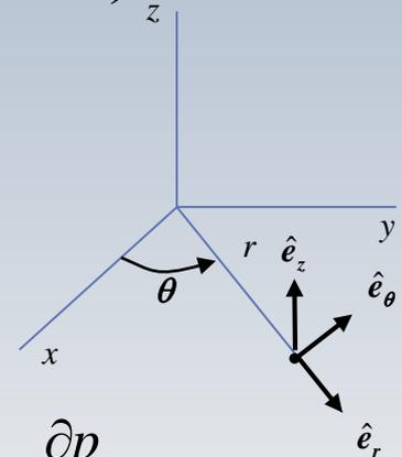
$$\frac{\partial p}{\partial r} = \rho r \omega^2 \quad \frac{\partial p}{\partial \theta} = 0 \quad \frac{\partial p}{\partial z} = -\rho g$$
