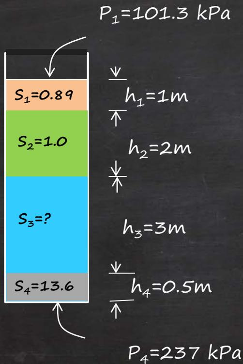
$$p_1 + S_1 \gamma_w h_1 + S_2 \gamma_w h_2 + S_3 \gamma_w h_3 + S_4 \gamma_w h_4 = p_4$$
